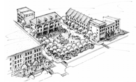
An "outdoor room" is created by surrounding an open plaza or greenspace with buildings.
