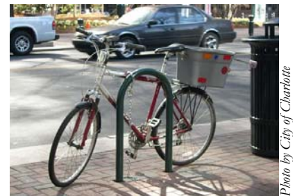
Example of an “Inverted U” bicycle rack. This rack will hold two bikes.
